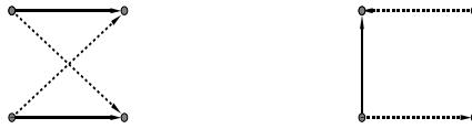
FIGURE 3.4. A sequence of two moves on 4 nodes: dashed edges are replaced by full edges.
